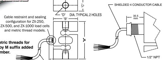
Also available with metric threads for most sizes. Designated by M suffix added to model number.
