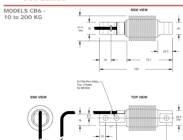
**IMPORTANT NOTICE**Dimensions are in mm unless noted otherwise. Request certified drawings before designing fixtures.
