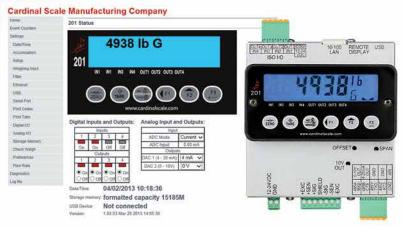
Connect the Ethernet port, enter the IP address in a Web browser, and the 201 transmitter will display live weight.
